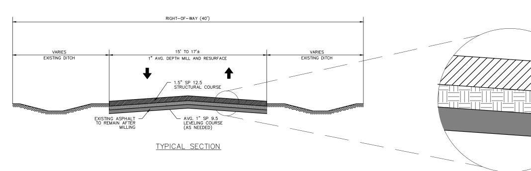
BASE MATERIAL MAY BE EXPOSED DURING MILLING OPERATIONS. IF ENCOUNTERED, CONTRACTOR IS RESPONSIBLE FOR PROVIDING PRIME AND TACK COATS PRIOR TO PAVING.
